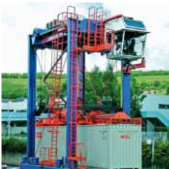
Straddle carrier made by Noell Mobile Systems are used as transport vehicles in container ports.
